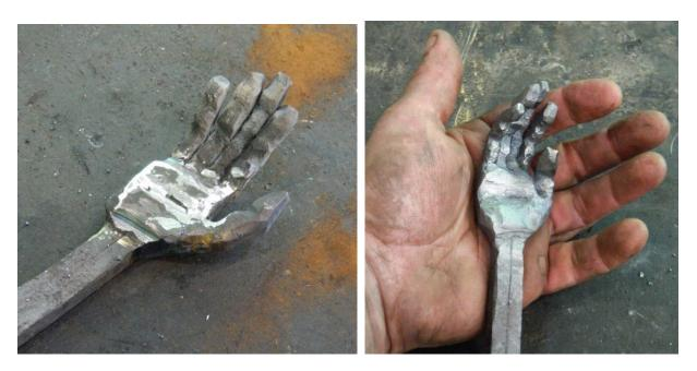
All welded. Then I took a good welding heat to stick it all together good, and then a few heats to dress and tinker with bends.
