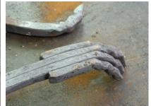
Four fingers tacked together and then lightly forge-welded
