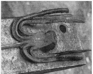
2. Punch the eyes with a 1/2" hollow point punch, and cross-hatch using a small chisel
