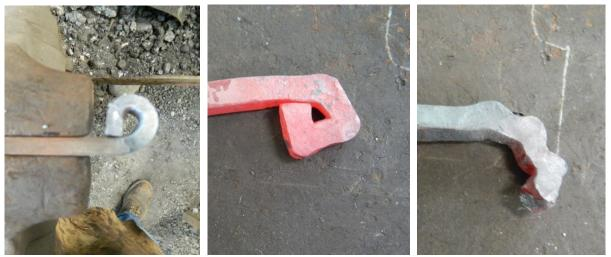
For each finger- a quick loop in 5/16 square bar. Square up the loop Open the loop
