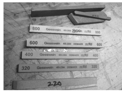
Started with 220 grit, then went to 320, 400, 600, and last an 800 stone
