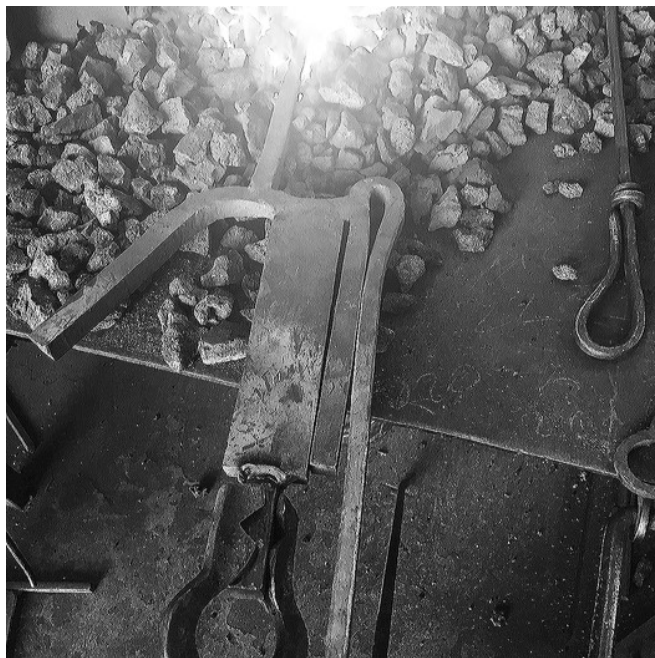
Get inner tine on the other side straight.
