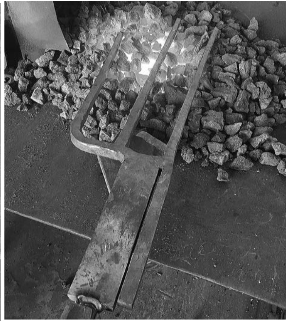
Bring outer tine around and straighten. Do the same on the initial side.
