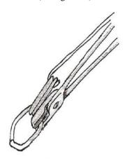
Figure 14: Holding the three links together for welding
