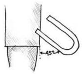
Figure 9: Starting the scarf of a chain link
