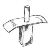
Braze or weld the square stock to the middle of the 1" flat stock. Mark & drill a 3/8" hole so when it passes through the flat stock it will be centered in the 1" square stock. Drill 3/4" deep. Place the vise pin holder in your vise and hammer the flat tabs to conform to the jaws. In a vise the pair of pin holders can be easily moved and secured in the position you need.
