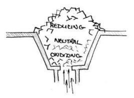
The "Oven effect" is achieved by making sure your pieces are covered in the fire. And it really doesn't take much for the oven effect to impact the welding process.
