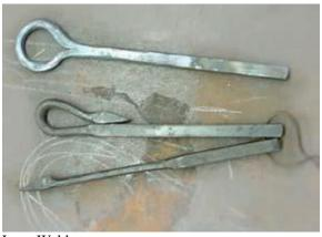
Loop Weld Commercial fluxes: http://www.superiorflux.com/welding.html manufacturer of EZWeld, Crescent Weld, and others.
