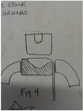
petal over the radius end of the mandrel and rotate in the vise as you bend the other petals. The mandrel is made of a 3" section of 1 ½" round. One end is left flat and the other is milled with a smooth radius to aid in forming the bottom of the tulip flower. The pattern is held in place using a ¼" rivet on the radius end. This step is done cold.
