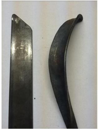
17. Heat each leaf and place in a bottom swage. Use the cross peen of the hammer to round and contour the entire length of the leaf. As your swage the center of the leaf pull the base of the leaf down to give it a gradually curve. This will allow the leaves to fall away from the stem of the flower. The base of the leaves will need to be rounded more tightly. This will make a more snug fit around the stem. Clean and smooth the base of each leaf with a grinder and wire brush.
