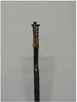
10. The Stems: Cut two sections of ¼" round stock at different lengths to be used as the flower stems (12"-14" sections). Use different lengths of stock if you would like for one tulip to be a little taller than the other. Grind the tips of each stem to look like a bluntly sharpened pencil. This will leave room for the weld when attaching the stamen to the stem.
