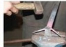
Photo 14 - Backing up the hammer blows with a pipe - a better choice than the horn
