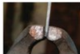
Photo 9 - Proper position for the start of the convenience bend
