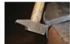
Photo 6 - Bend without necking down the base of the taper
