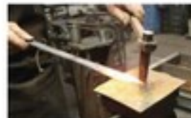
Photo 3 - Hot cutting using a treadle hammer
