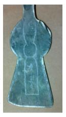
One the widening of the spatula and spoon, Shel pointed out (as did Peter Ross at Madison) that the peen of the crosspeen hammer should be flat and wide with beveled edges, like the face. This will cause the metal to move away from the center easier than with a rounder, pointier peen (Mark Aspery's cow poop theory) and the result will be a smoother, more uniform finish. Have you noticed that these instructors we bring to you know a lot of neat stuff?
