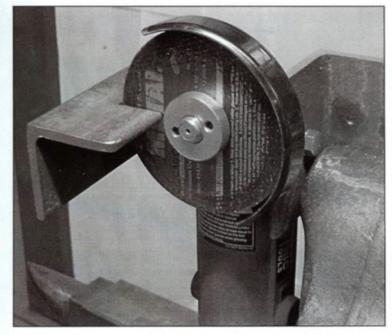
To make the leaves, I made a pattern out of 16 gauge steel. Using this pattern, I traced the outline onto the sheet steel. Then I rough sheared the blank out with a plate shear. Moving over to the mini abrasive-wheel table saw, I followed the scribed lines of the leaf. Go slowly. The wheel can be very aggressive and can cut quickly. Next, wire brush the burrs and touch up with a file. I then used my veining tool to give the leaf some character.
