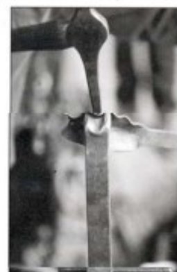
Leafing hammer and swage at work.
