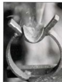
Scooping the leaf in a 45° swage designed to be used in a vise.
